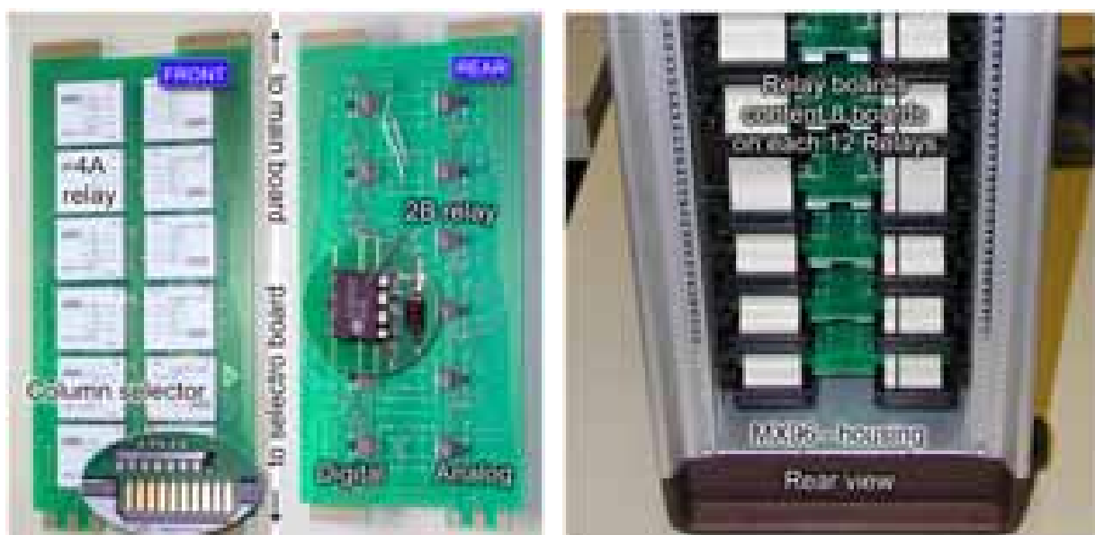
Fig. 34. Relay board PCB front and rear view (left), placement of relay boards in MX96 – rear view (right)
