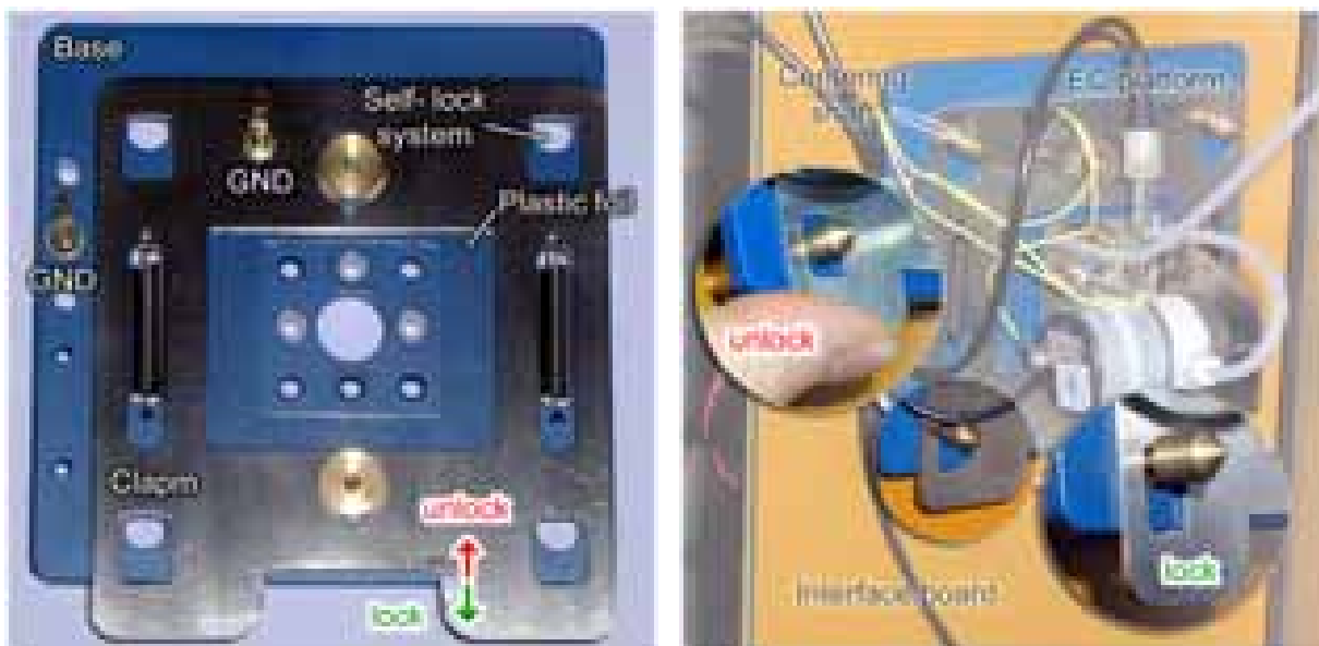
Fig. 12. Self-locking mechanism of the EC platform (left), EC platform locked in the EC set-up, principle (right)
