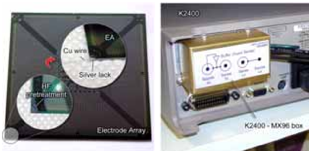
Fig. 30. Electrical connection to the semi-conducting support of the EA (left), K2400-MX96 shielding box (right)
