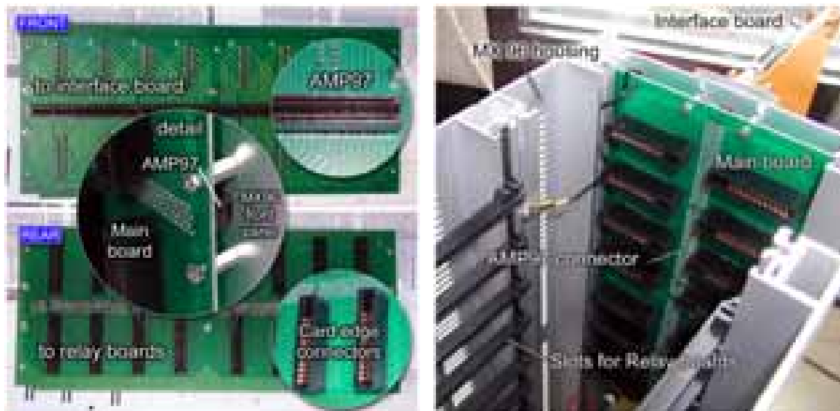
Fig. 33. MX96 main board PCB front and rear sides (left), its implementation into the MX96 housing with the plugged-in interface board (right)
