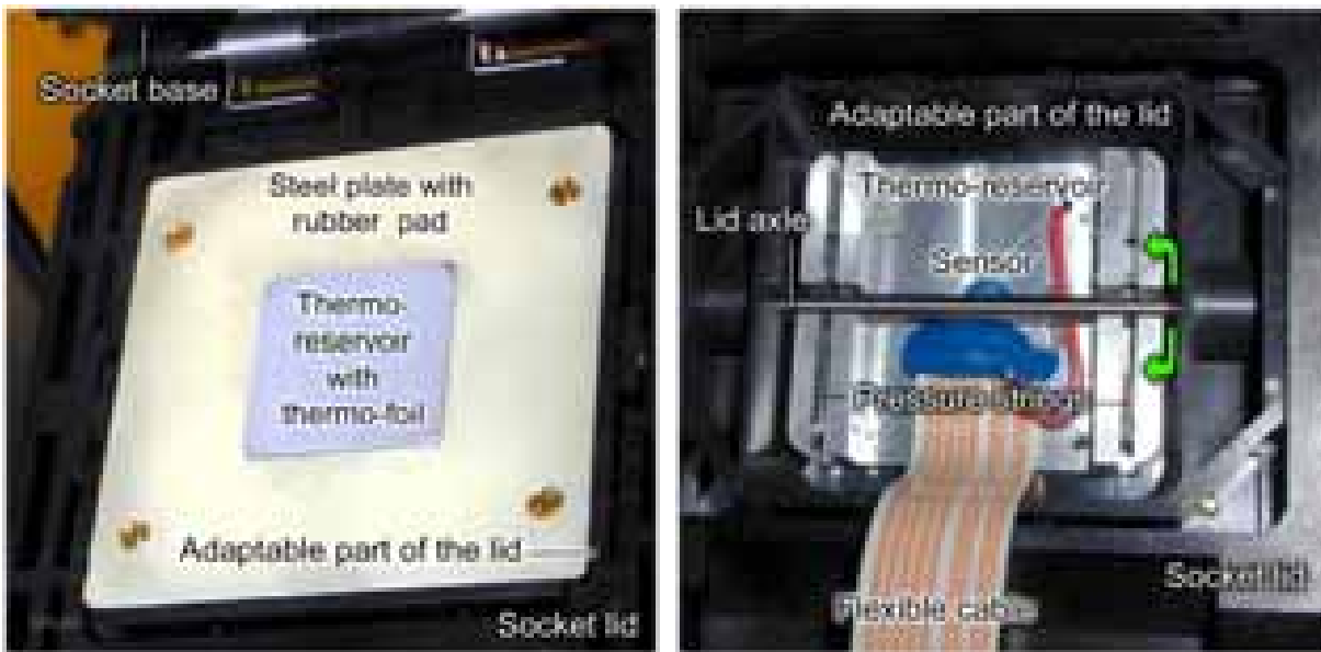
Fig. 42. Front view of the socket lid with adaptable part and the thermo-reservoir (left), rear view of the thermo-reservoir fixed to the adaptable part of the socket lid (right)
