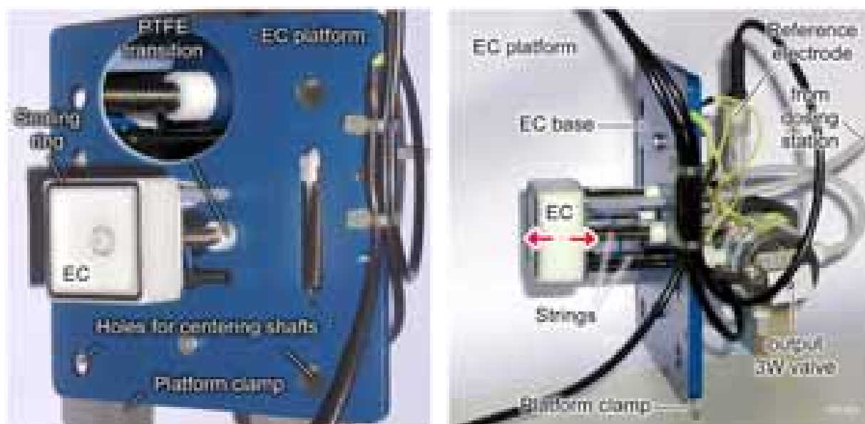
Fig. 13. Front view of the EC platform with the electrochemical cell body (left), side view of the EC platform with outlined one-way movement of the EC (right)
