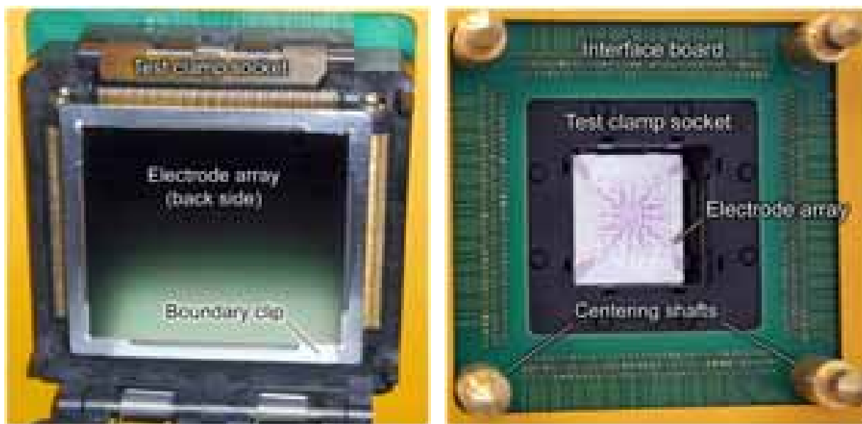
Fig. 25. Detailed view of the interface board, front view with the inserted electrode array (left) and rear view with attached electrode array without electrochemical cell (right)
