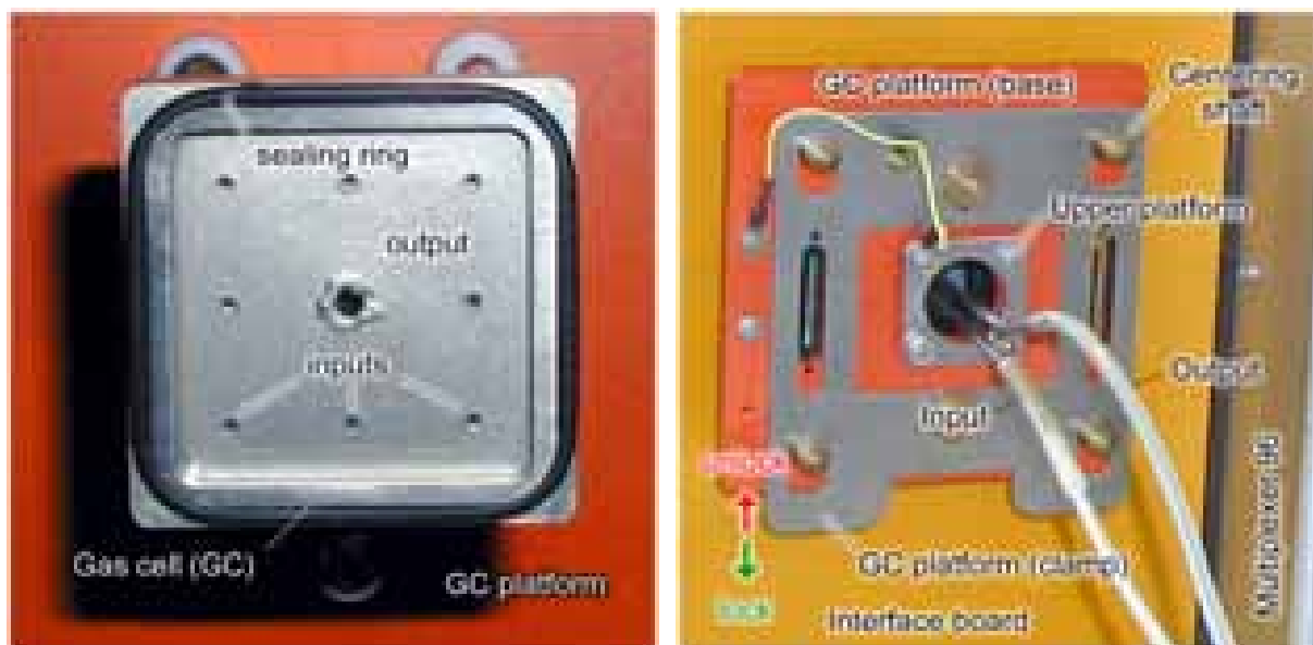
Fig. 68 Gas cell – front view (left), self-locking mechanism of the gas cell platform (right)
