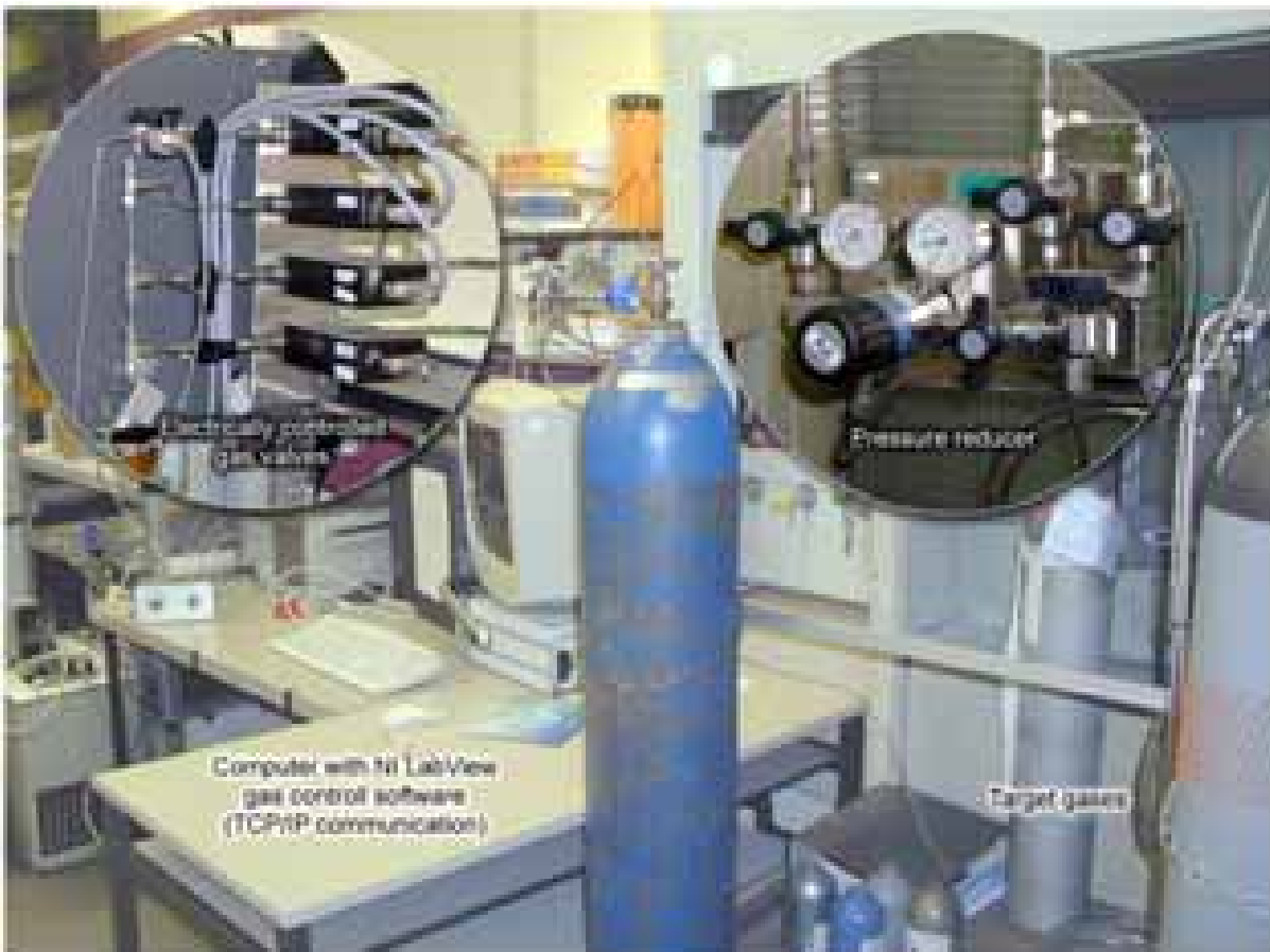
Fig. 67. Practical realization of the gas flow system
