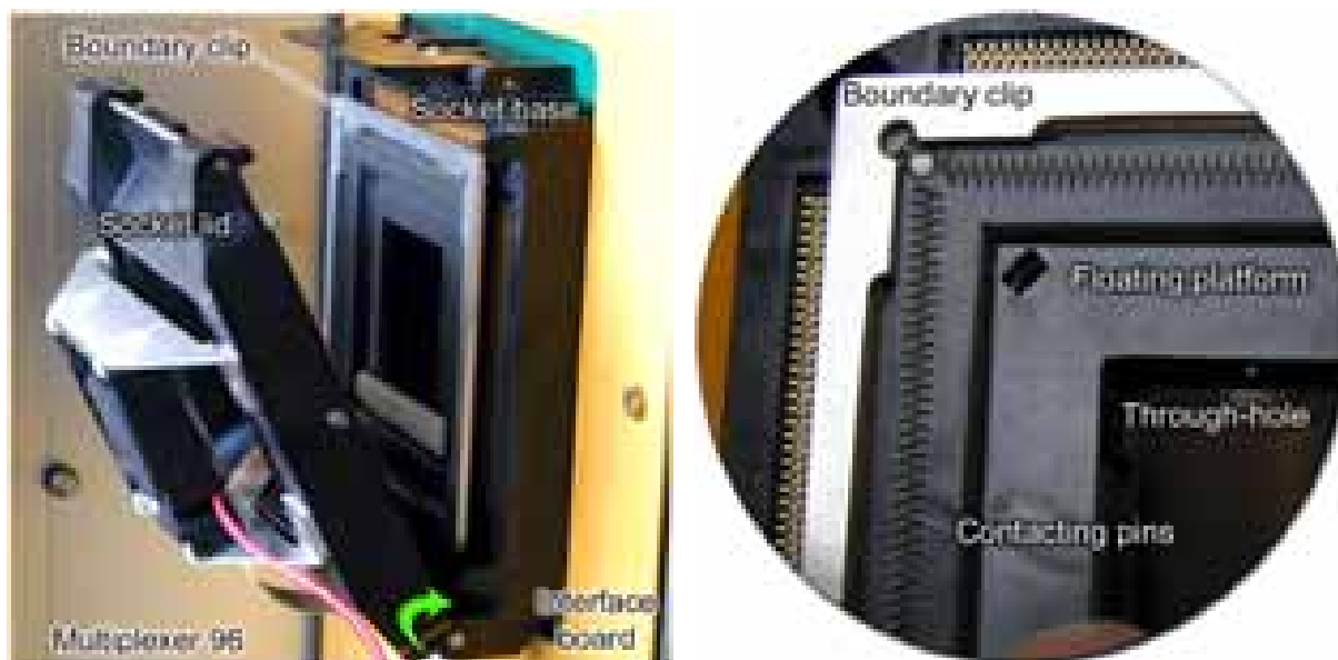
Fig. 24. Test clamp socket (left), detailed view of contact pins of the socket (right).
